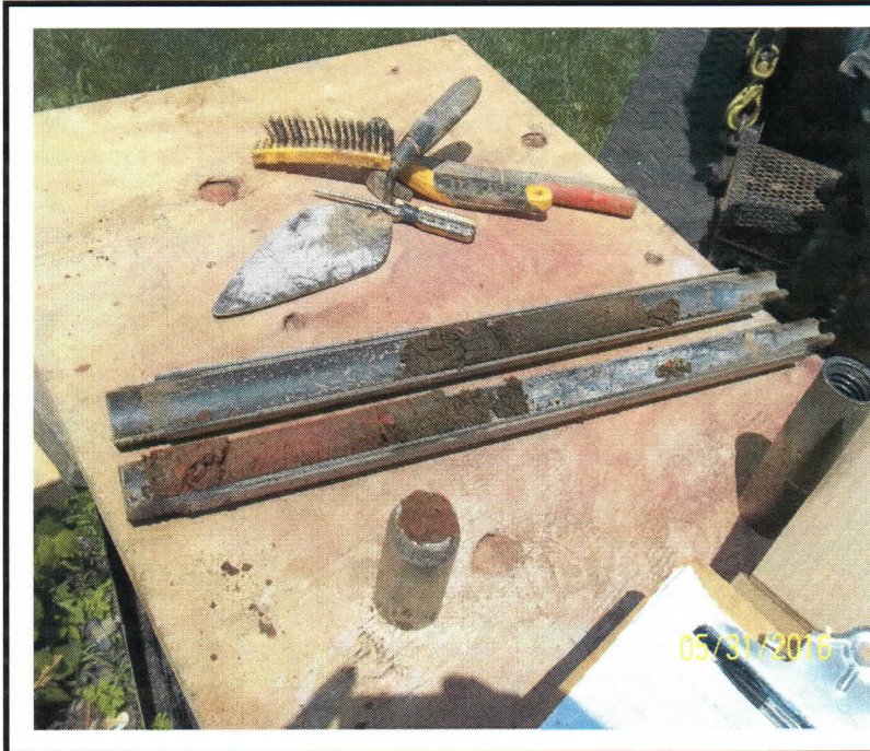
Sample recovery from split spoon samplers
