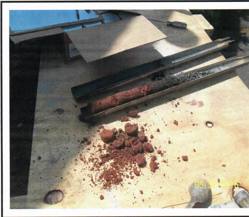
Sample recovery from split spoon samplers
