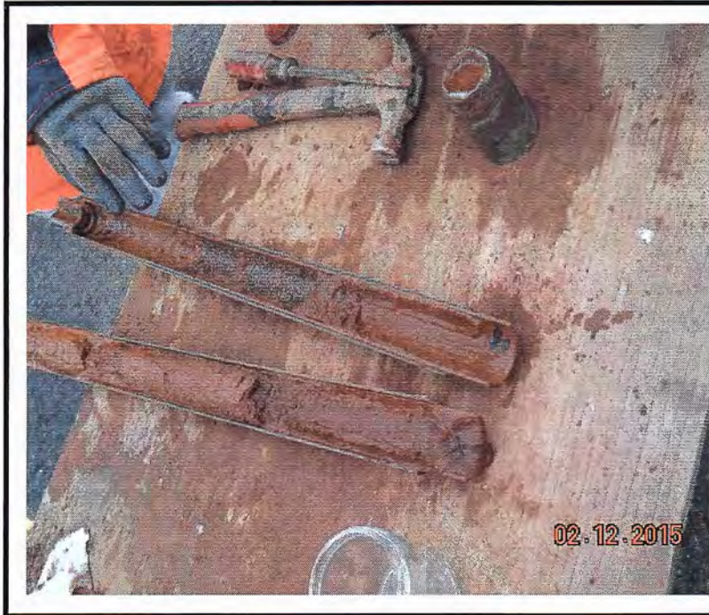
Sample recovery from split spoon samplers
