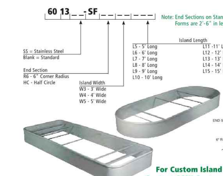
1.08 DTL2 ISLAND FORM DETAIL NOT TO SCALE
