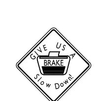
36" x 36" (9 S.F.) NOTE: THE BORDER, THE WORDS "GIVE US A ", "SLOW DOWN!, AND THE BRAKE PEDAL ARE BLACK; LEAVING THE WORD "BRAKE" ORANGE
