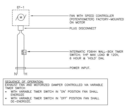
2 EXHAUST FAN WIRING SCHEMATIC
