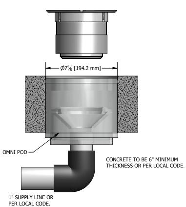
SUPPLY LINE TO BE SOLVENT WELDED TO
