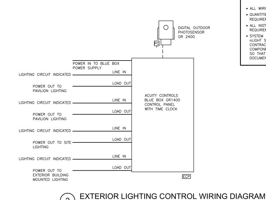
• ALL WIRING SHALL BE AS PER MANUFACTURER REQUIREMENTS • QUANTITIES OF ALL DEVICES SHALL BE AS PER MANUFACTURER REQUIREMENTS/RECOMMENDATIONS • ALL INSTALLATIONS SHALL BE AS PER MANUFACTURER REQUIREMENTS • SYSTEM DESIGN AND LAYOUT IS BASED ON ACUITY CONTROL nLIGHT SYSTEM. IF SYSTEM IS SUBSTITUTED, IT IS THE CONTRACTORS RESPONSIBILITY TO PROVIDE ALL REQUIRED COMPONENTS, SOFTWARE AND NETWORK CONNECTIONS REQUIRED SO THAT SYSTEM OPERATES AS INDICATED ON CONSTRUCTION
