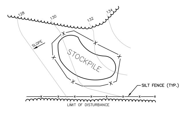
TOPSOIL STOCKPILE DETAIL.
