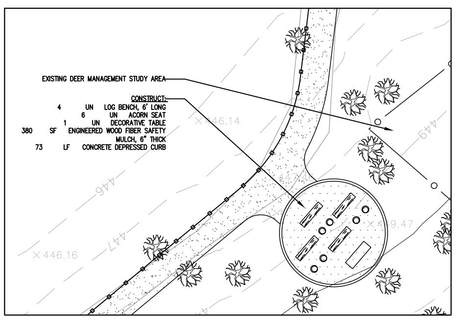
给 UN LOG BENCH, 6' LONG UN ACORN\_SÉAT UN DECORATIVE TABLE UN FIRE WOOD STORAGE RACK WITH COVER SF ENGINEERED WOOD FIBER SAFETY MULCH, 6" THICK LE CONCRETE DEPRESSED CURB  $\times 425.37$
