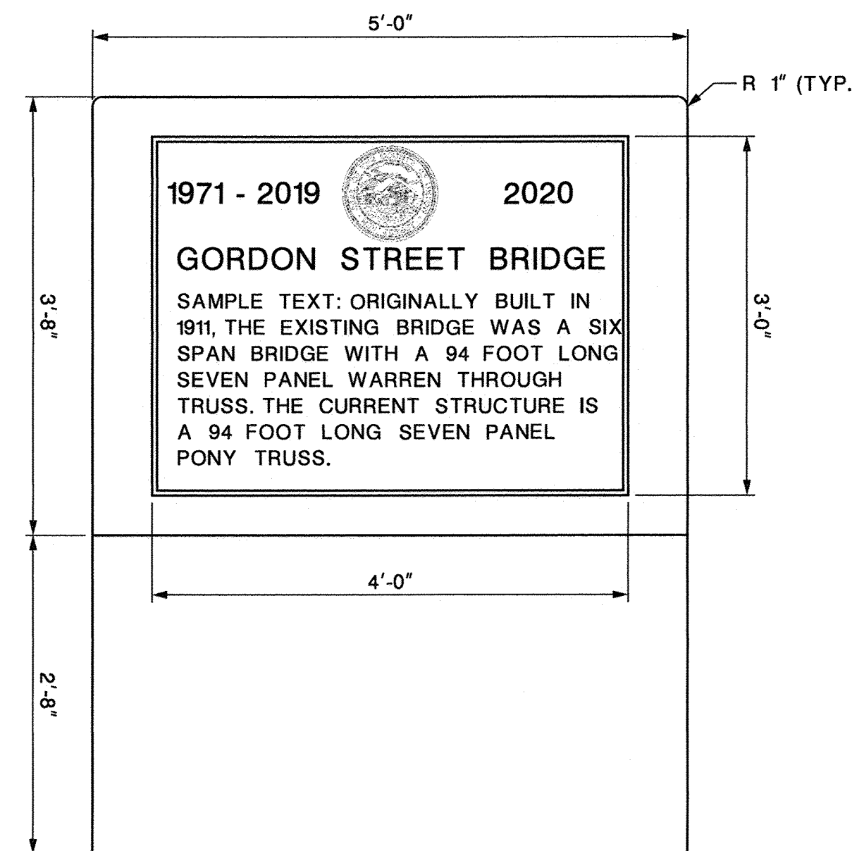
SPECIALIZED SIGN DETAIL APPROACH SPAN SCALE: 1/2" = 1'-0"
