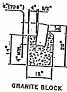
CROSS SECTION STANDARD HEIGHT CURB
